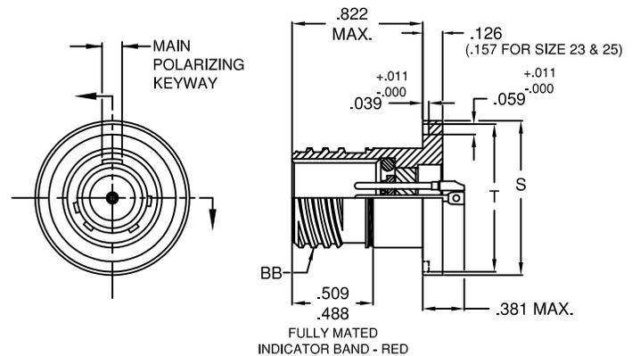
\*- : Z1= CRES SHELL, PASSIVATED; Z2= CRES SHELL, ELECTRODEPOSITED NICKEL; Z3= CRES SHELL, CADMIUM WITH OLIVE DRAB.
